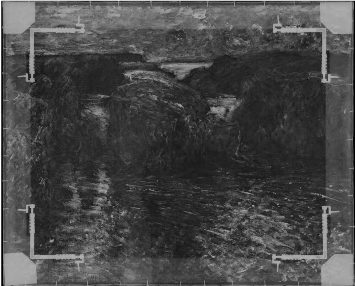
Figure 1: Composite x-ray created by Professor Erdmann's stitching software for the entire painting.
