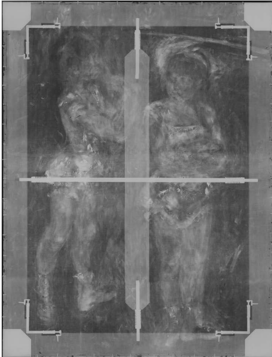
Figure 1: Composite x-ray created by Professor Erdmann's stitching software for the entire painting.
