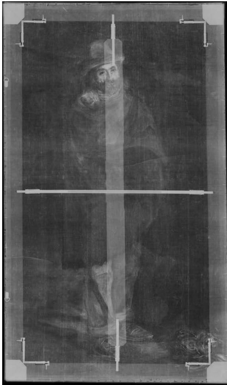
Figure 1: Composite x-ray created by Professor Erdmann's stitching software.
